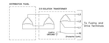
Figure 9: Delta to Delta Isolation Transformer
